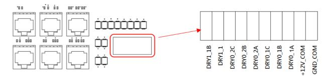
DRY1 1B/DRY1 1: Used to start the driver.
