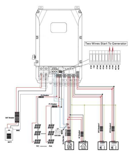
8.1.2. The Generator is normally connected to the Generator port. The connecting cable between the Generator and the inverter does not need to be covered with CT. The connection line of the power grid port should be connected with CT. The system diagram is as follows.
