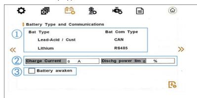
(1) Set Battery Type and Battery Communication method
