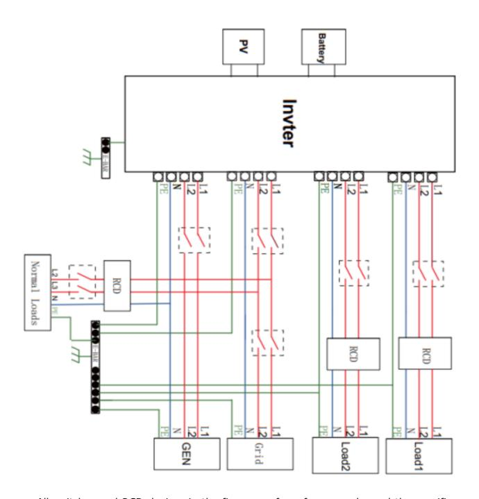
All switches and RCD devices in the figure are for reference only, and the specific installation shall be subject to local regulations.
