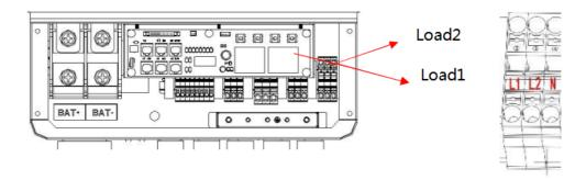
Inside the inverter, load2 is connected to load1 through a relay, and the relay disconnect when the SOC of battery is lower than set value. At this time, the load2 is powered off and load1 is still powered on. (The total power of Load1 plus Load2 should not more than the rated BACK-UP power when GRID is off)
