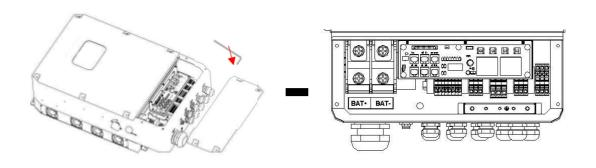
**Step 5**: Pass the corresponding conduit and fasten the joint.
