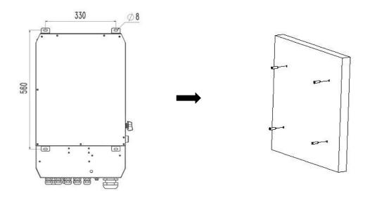
**Step 2**: Lift up the inverter and align the hole of the inverter with the expansion bolt, fix the inverter on the wall.
