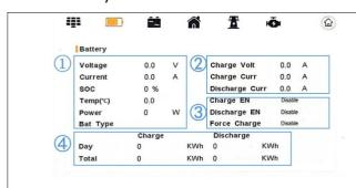
(1) Display the working parameters of the battery, including real-time voltage, real-time current, battery surplus capacity, battery temperature, battery power, and battery type.
