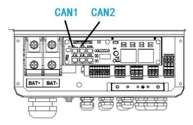
For parallel communication, CAT 5 cables are needed. The units should be connected hand by hand.
