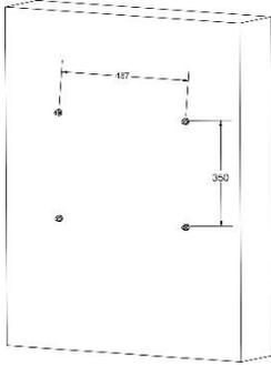
2. Raise the inverter and place it over the four screws.
