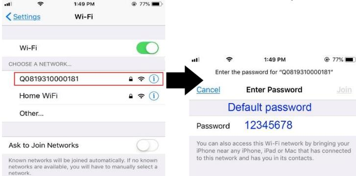
Then, return to WatchPower APP and tap “ **Confirm Connected Wi-Fi Module** ” button when Wi-Fi module is connected successfully.
