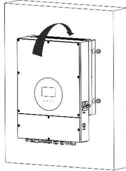
3. Check if the inverter is firmly secured.
