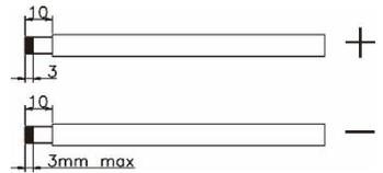
The cable size of each inverter is shown as below:
