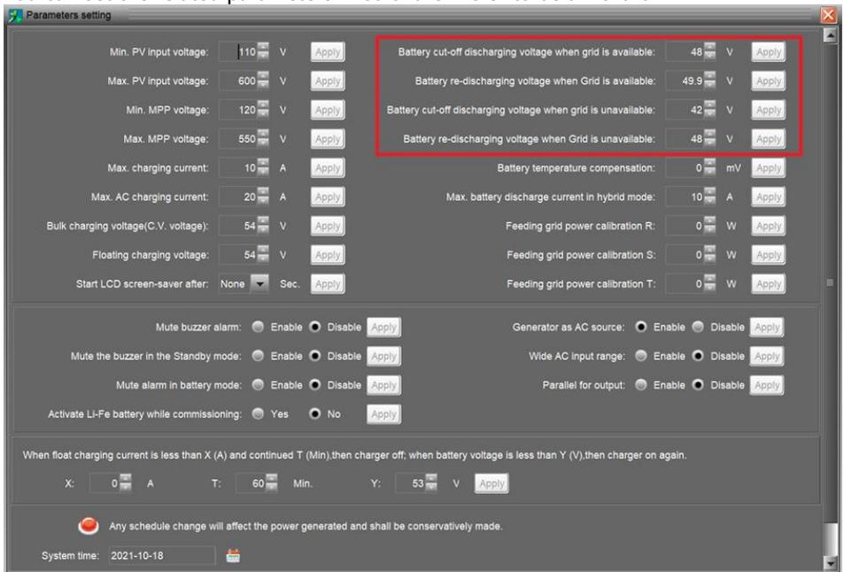
The screenshot shows the 'Parameters setting' window with various configuration options. A red box highlights the following parameters:
