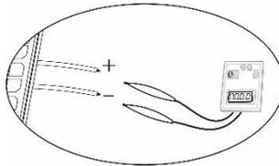
**CAUTION:** Exceeding the maximum input voltage can destroy the unit!! Check the system before wire connection.
