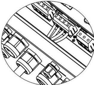
The reference tightening torque is 1.0-1.5 N.m.
