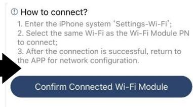
Enter the "Settings→Wi-Fi" and select connected Wi-Fi name. The connected Wi-Fi name is the same to your Wi-Fi PN number and enter default password "12345678".
