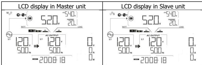
Step 5: If there is no more fault alarm, the parallel system is completely installed.
