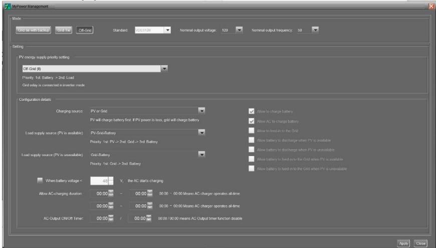
**PV energy supply priority setting: 1<sup>st</sup> Battery, 2<sup>nd</sup> Load**
