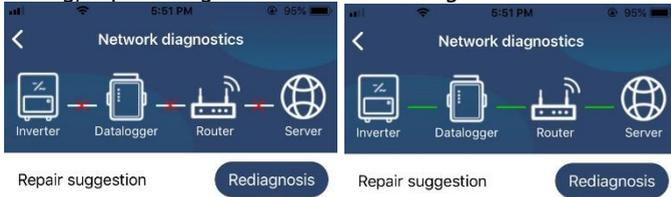
**The Inverter and the datalogger communicate abnormally.**
