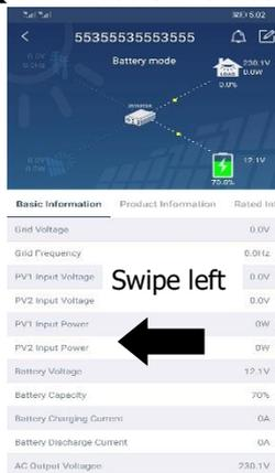
**【Basic Information】** displays basic information of the inverter, including AC voltage, AC frequency, PV input voltage, Battery voltage, Battery capacity, Charging current, Discharging current, Output voltage, Output frequency, Output apparent power, Output active power and Load percent. Please slide up to see more basic information.
