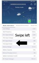
**[Basic Information]** displays basic information of the inverter, including AC voltage, AC frequency, PV input voltage, Battery voltage, Battery capacity, Charging current, Discharging current, Output voltage, Output frequency, Output apparent power, Output active power and Load percent. Please slide up to see more basic information.
