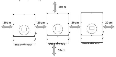
**NOTE:** For proper air circulation to dissipate heat, it's necessary to allow a clearance of approx. 20 cm to the side and approx. 50 cm above and below the unit. Be sure to install each unit in the same level.
