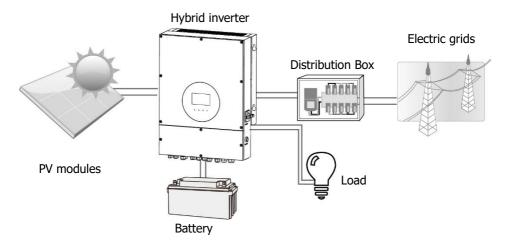
Figure 1 Basic hybrid PV System Overview
