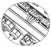
The reference tightening torque is 1.0-1.5 N.m.
