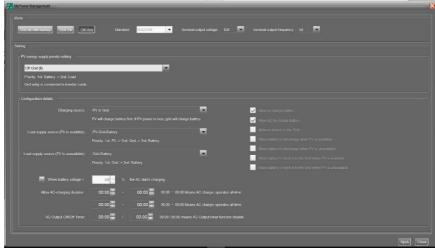
PV energy supply priority setting: 1st Battery, 2nd Load
