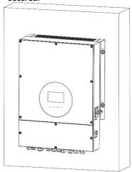
2. Raise the inverter and place it over the four screws.
