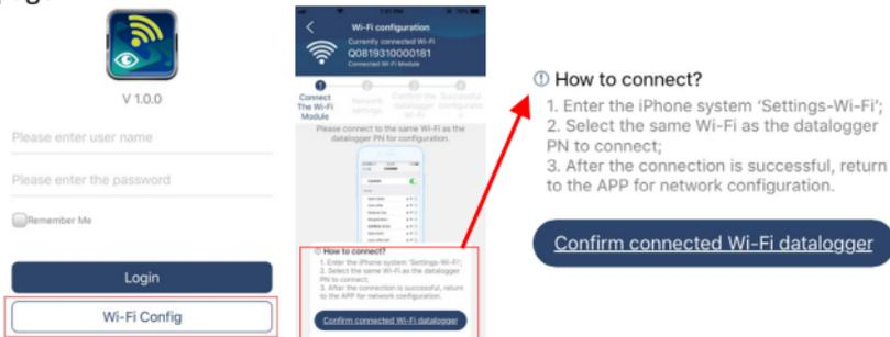
**Step 2:** Follow How to connect instruction, switch mobile phone page to Wi-Fi list. Find the Wi-Fi PN number(Q08XXXXXXXXXXXX) of your Wi-Fi module in accordance with Network name to connect by entering default password: 12345678. Then return to Wi-Fi configuration page when connected successfully.
