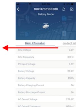
**【Basic Information】** displays basic information of the inverter, including AC voltage, AC frequency, PV input voltage, Battery voltage, Battery capacity, Charging current, Output voltage, Output frequency, Output apparent power, Output active power and Load percent. Please slide up to see more basic information.
